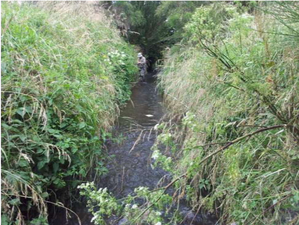
Photo 17: Stu carrying out the habitat survey on a North Head Stream control site. Note the white tile in the centre of the picture that was used for the shuffle test; a metric of fine sediment deposition.
