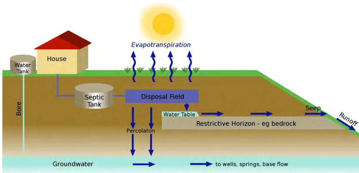
**Figure 3: Flows of wastewater to and from a disposal field**
